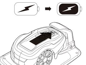
Place the mower into the charging station while the boundary and guide wires are being laid.
