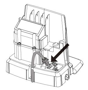
Connect the low voltage cable to the charging station.
