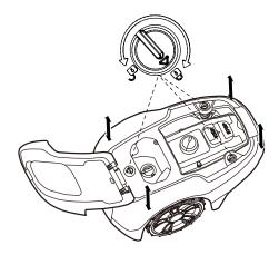
Rotate the knob to the unlock position and lift firmly at one of the corners of the body and repeat for all four corners, until the body pops loose from the chassis.
