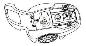
Press the STOP button on the mower and remove the safety key.
