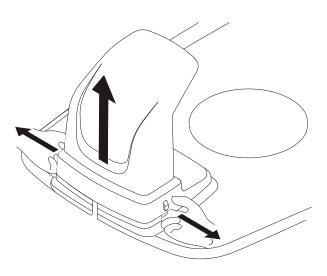
Remove the protective cover on the charging station by pressing in the tabs on each side of the base and lifting away the cover.
