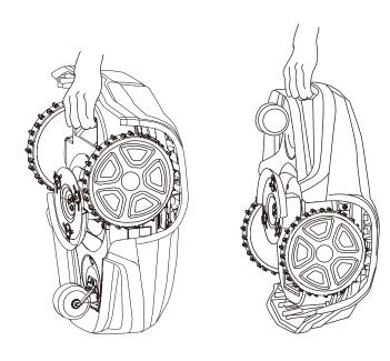
Press the **STOP** button and remove the safety key before lifting. Always lift the mower using the carrying handle.
